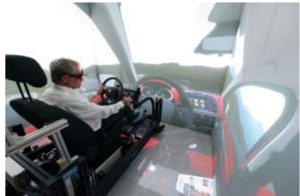
Figure 5. Renault's high performance CAVE™ with driver station
