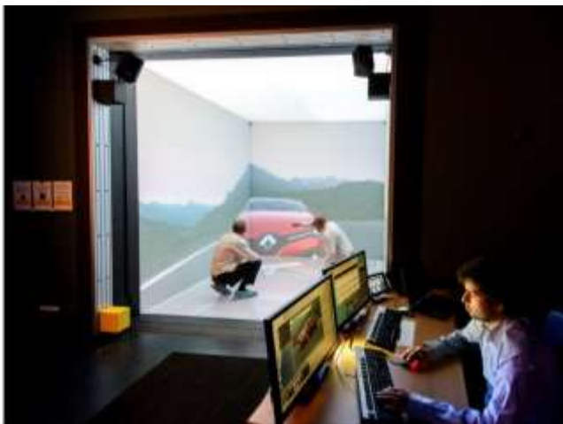
Figure 3. Renault's 70 M 3D pixels 5 – sided high performance CAVE™
