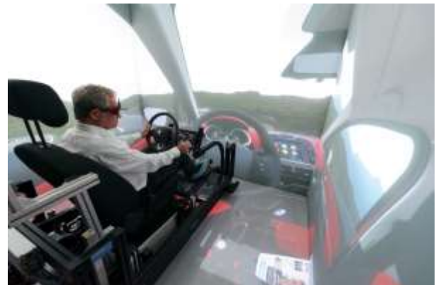
Figure 5. Renault's high performance CAVE™ with driver station
