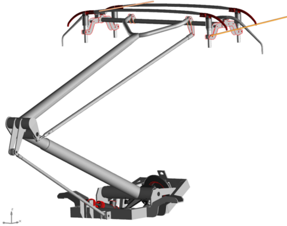
Figure 5 – Multibody pantograph: overhead crossing simulation
