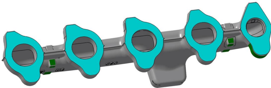
Fig. 1: CAD representation of the part for the specified operation (5 machined flanges in blue, reference surfaces in green)
