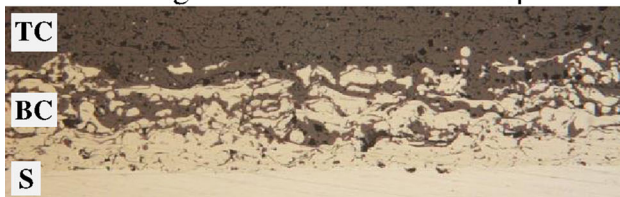
Plasma graded BC: thickness 280μm
