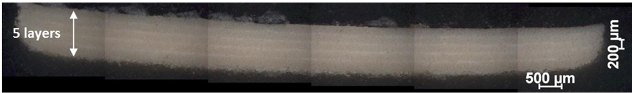
Figure 17 : Cross section of a squared PA12 sample obtained with 5 additive layers, ( T_0=440 K, P=1.6 W, V= 0.2 m/s). Fused layer thickness h is near 150 \mu\text{m} , and a -z shift of -120 \mu\text{m} of the building plateau has been used to carry out additive layers.
