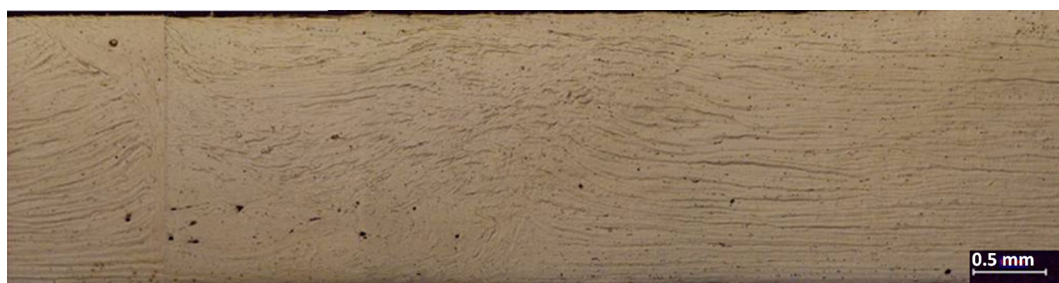
Fig. 4—Macrostructure of FSW cross-section showing shear bands on both weld sides.
