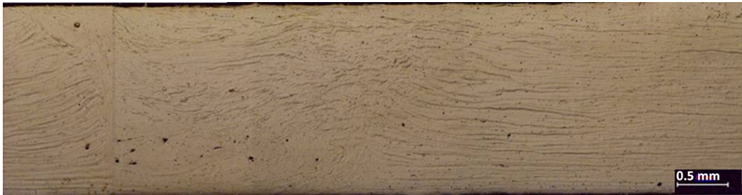
Fig. 4—Macrostructure of FSW cross-section showing shear bands on both weld sides.
