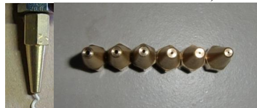
Fig 9. 3D Printing head's nozzles
