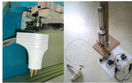
Fig 8. 3D Printing head on NC, and the piston depositing.
