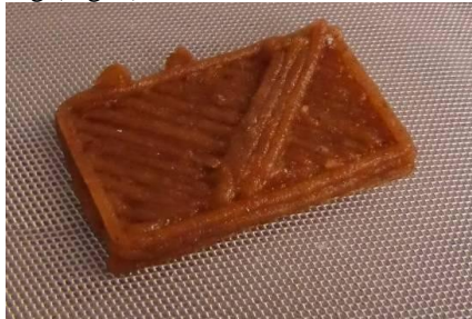
Fig 3. First reconstituted wood model by additive manufacturing
