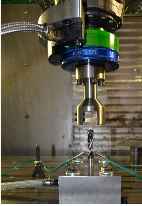
Fig. 4 Experimental set-up for temperature measurement
