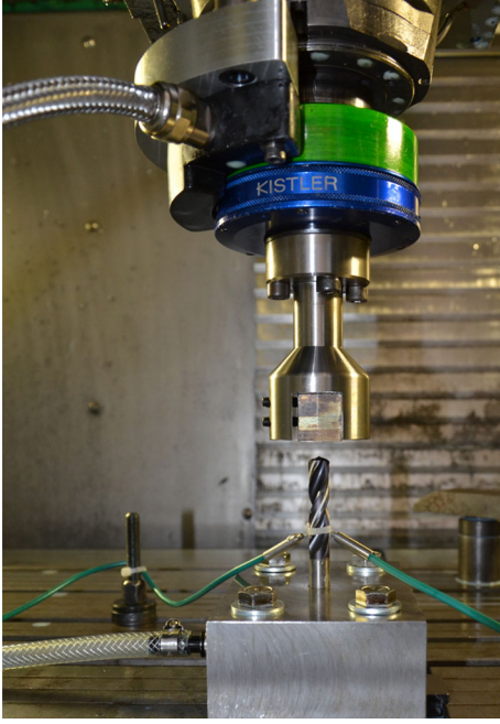
Fig. 4 Experimental set-up for temperature measurement
