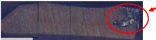
Figure 17 : Tool wear measurement
