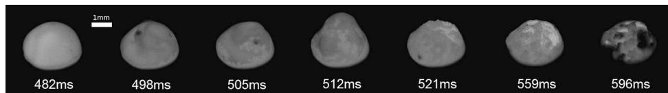
Fig. 7 Cooling liquid oxide melt on the top of a pure iron rod (P(angle of view 45°), laser initiation: 320 W–300 ms) - An oxygen bubble is about to burst at t = 512\text{ ms}
