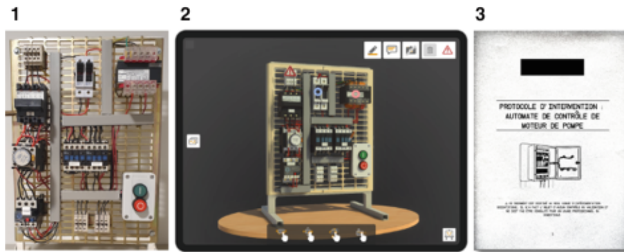
Fig. 2. From left to right: 1. The electrical panel on which the maintenance operation is to be performed. 2. The telecollaboration application on the Tab S7 + 5G tablet. 3. The manual detailing the maintenance procedure.
