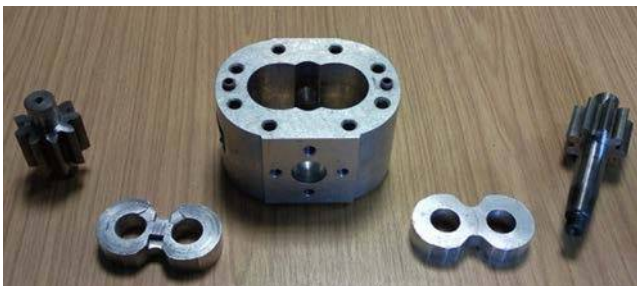
Figure 7 Real gear oil pump components
