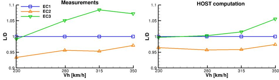
Figure 2: Forward flight performance for three blades, expressed in terms of the normalized aerodynamic efficiency  $L/D$ , versus the forward flight velocity. Left: wind tunnel measurements; right: HOST computations
