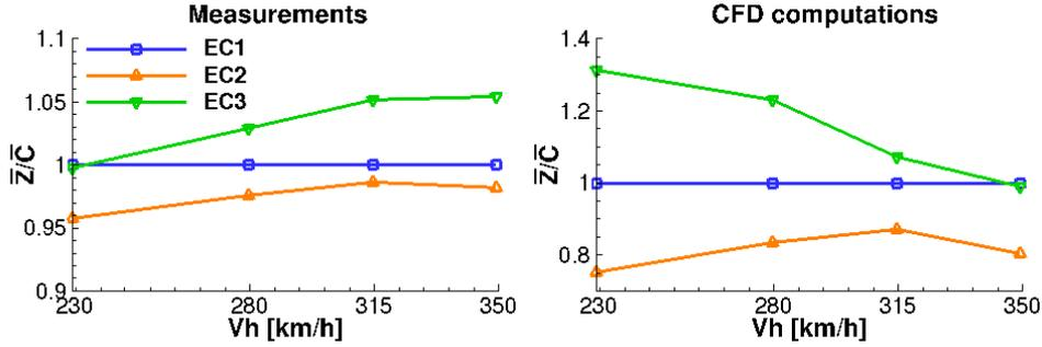
Figure 3: Forward flight performance for three blades, expressed in terms of the normalized  $\bar{Z}/\bar{C}$  ratio, versus the forward flight velocity. Left: wind tunnel measurements; right: CFD computations
