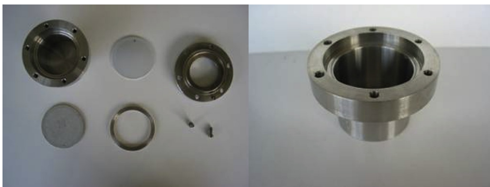
Fig. 1. Pictures of a liquid permeation cell.
