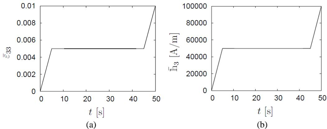
Figure 2: Macroscopic loading conditions for the composite: a) strain and b) magnetic field path.
