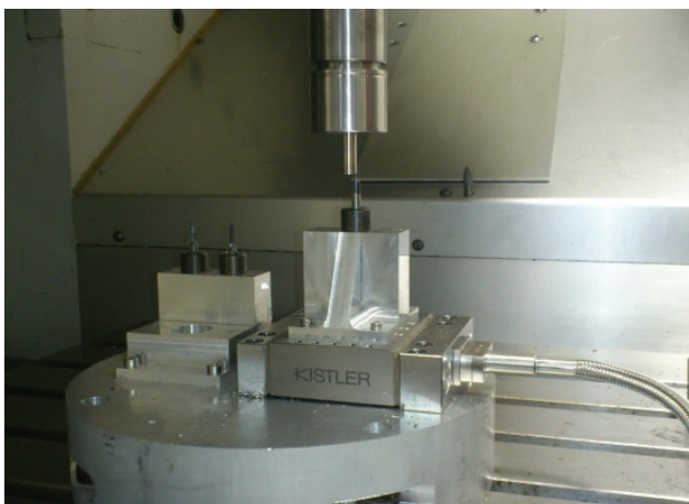
Fig 1: Micro-cutting experimental setup
