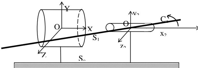
Figure 16. Displacements of the shaft after loading
