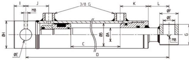
Figure 12. Hydraulic tube with two cylindrical joint
