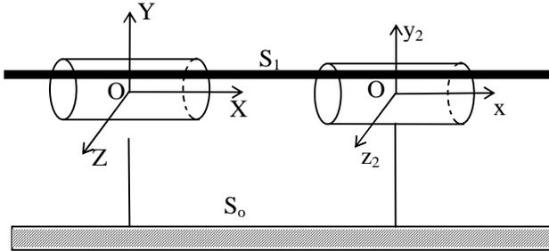
Figure 14. Displacement of the shaft after loading
