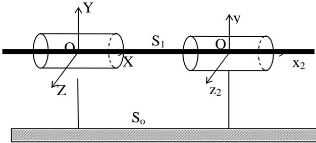
Figure 13. Clearance model of two cylindrical joints
