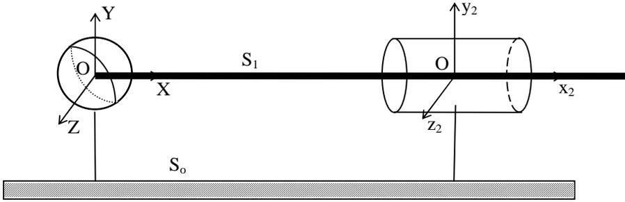
Figure 4. Clearance model of spherical and cylindrical joints
