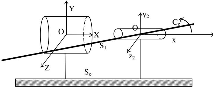
Figure 15. Displacements of the shaft after loading
