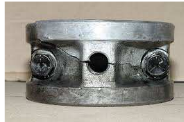
Fig.1. Failure of circular cylindrical bearing
