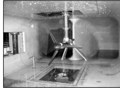
Fig. 6. The tested marine turbine [27].
