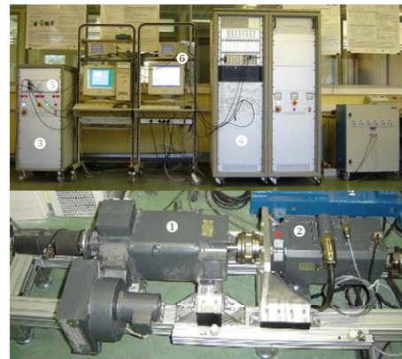
Fig. 13. Components of the G2ELAB test bench, Grenoble, France: ① DC motor, ② PMSG, ③ Power electronics for driving the DC motor, ④ Power electronics for driving the PMSG, ⑤ DSP TMS320F240 implementing DC motor control, ⑥ DSP DS1005 (dSPACE) implementing PMSG-based MCT control.
