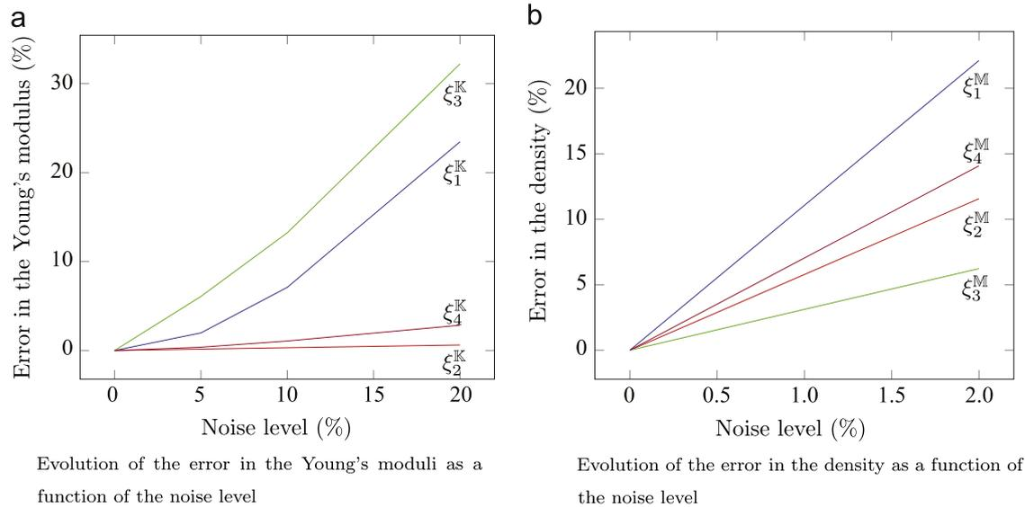
**Fig. 6.** Influence of the measurement noise level on the quality of the structural parameter estimations. (a) Evolution of the error in the Young's moduli as a function of the noise level. (b) Evolution of the error in the density as a function of the noise level.
