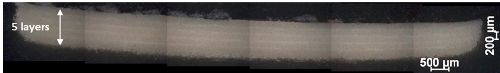
Fig. 17. Cross section of a squared PA12 sample obtained with five additive layers, ( T_0 = 440 \text{ K} , P = 1.6 \text{ W} , V = 0.2 \text{ m/s} ). Fused layer thickness h is near 150 \mu\text{m} , and a -z shift of -120 \mu\text{m} of the building plateau has been used to carry out additive layers.
