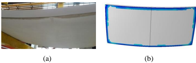
Figure 11. Contact zones on the lower part of the sheet, a- experimental result, b- numerical result
