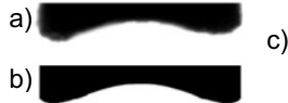
Fig.6. Tool profiles. a) Experimentation b) Simulation c) Profiles differences. black: simulation extra volume.
