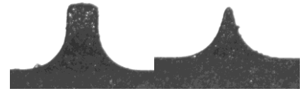
Fig. 5. Tungsten carbide tools after erosion
