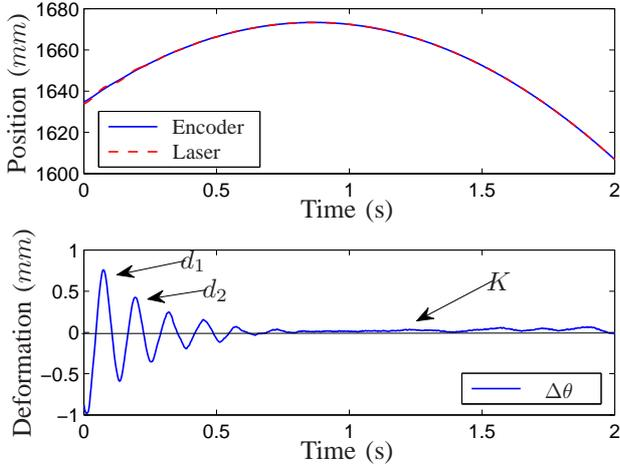
Fig. 4. Temporal evolution of the X position (top) and its deformation (bottom).
