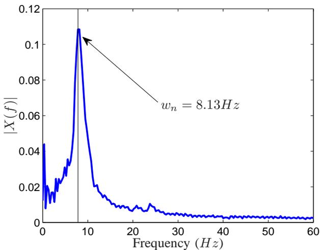
Fig. 5. Fourier transform of the X deformation.
