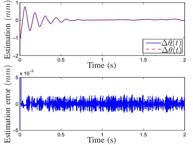
Fig. 6. Sliding mode deformation observation and its error.
