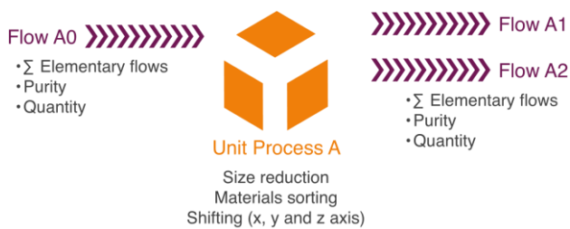
Fig. 2 Modelling of a recycling pathway step with a unit process and its related flows
