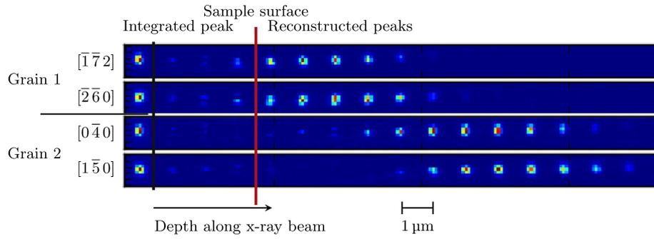
**Fig. 3.** Laue spots from two different Sn grains, reconstructed in depth along the X-ray beam. The red line indicates the sample surface. To the left the integrated peak is shown, i.e. the peak as measured by the detector when the W wire has been removed. (For interpretation of the references to color in this figure legend, the reader is referred to the web version of this article.)
