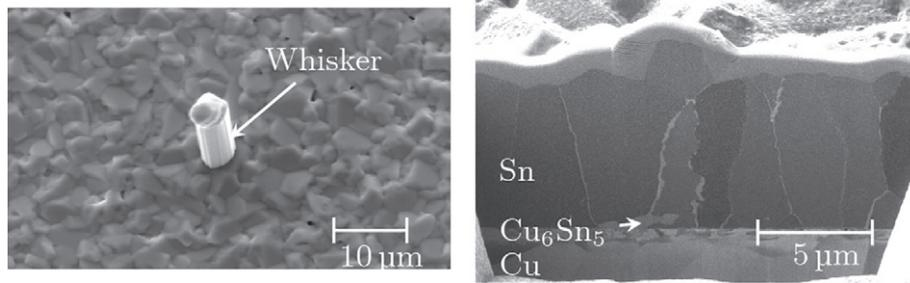
**Fig. 1.** Left: SEM image of the tin whisker selected for the microdiffraction measurements. Right: FIB cross section showing the columnar grain structure of the Sn layer and the formation of  $\text{Cu}_6\text{Sn}_5$  at the Cu-Sn interface and at grain boundaries between Sn grains.
