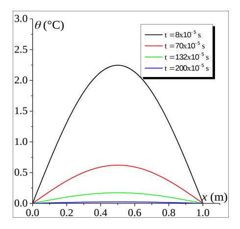
Figure 4: The temperature as a function of x at different times.
