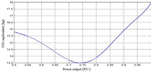
Fig. 5. CO<sub>2</sub> equivalent emission characteristic of MGT No2 (30kW)
