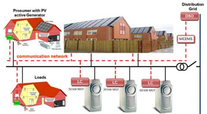
Fig. 11. Schematic diagram of the urban microgrid
