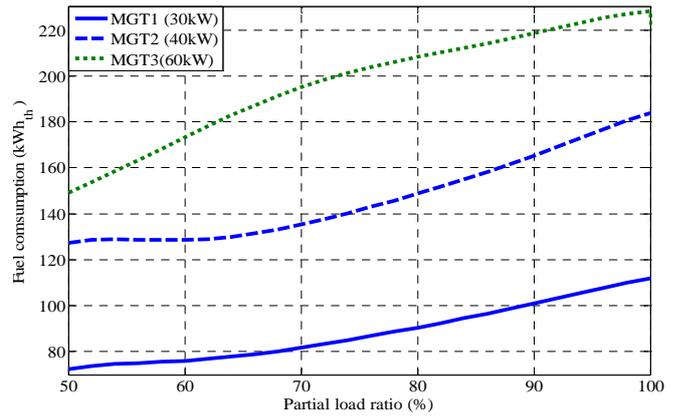
Fig. 4. Fuel power consumption of various MGT
