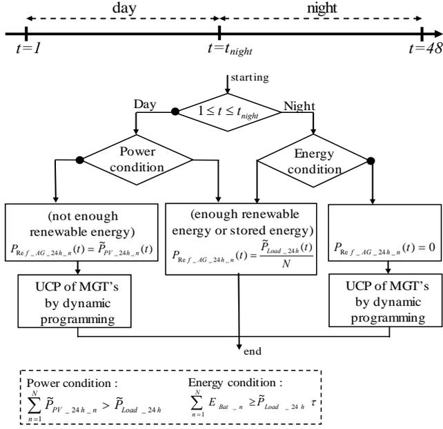
Fig. 8. Power reference calculation and dispatching.
