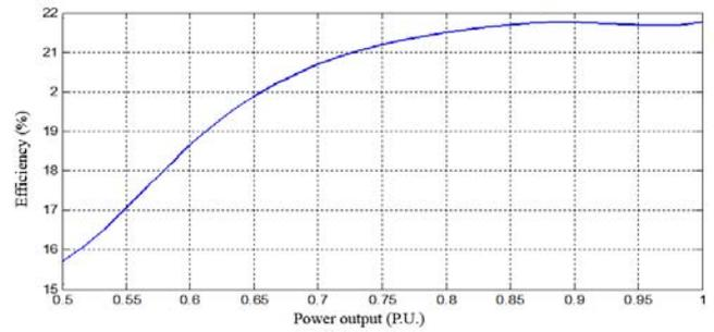
Fig. 3. Efficiency characteristic of MGT 2 (30kW)
