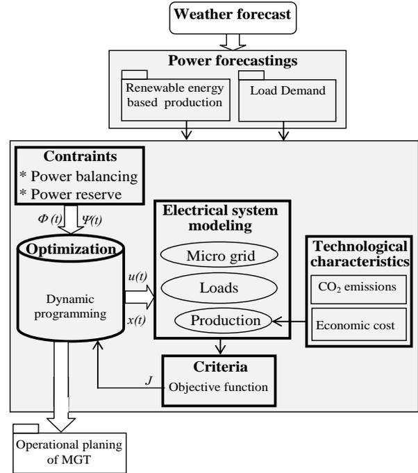
Fig. 6. Scheme of the day-ahead optimal operational planning
