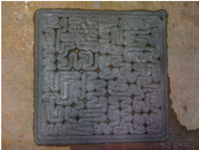
Fig. 8. The impact of nozzle direction changes on the layer density, causing underfill problems.
