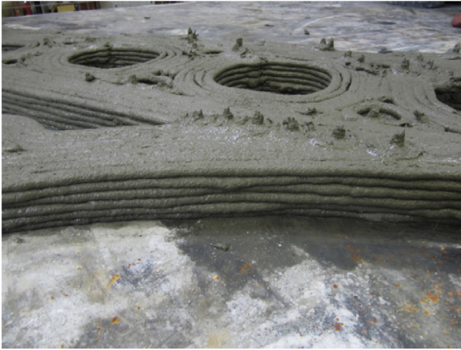
Fig. 11. The impact of nozzle start/stop operations on the deposited layer volume, causing overfill which contributes to deformation and conformity issues.
