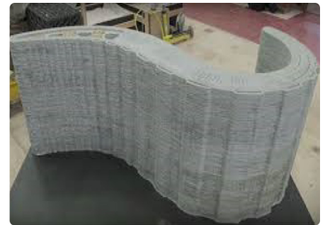
c) a solid geometry, vertically printed component. Image: Loughborough University, UK.
