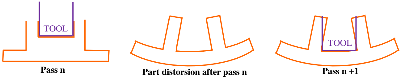
Figure 4: Sequence effect on stiffener sides
