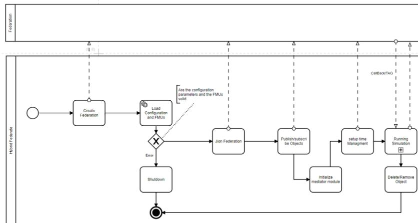
Figure 7: Lifecycle of the HLA Hybrid Federate.
