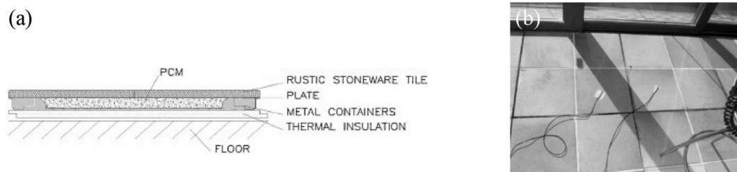
Fig. 19. (a) Cross section of the tile, and (b) Image of the tile installed onto the floor of the room [127]. Copyright (2019), with permission from Elsevier.
