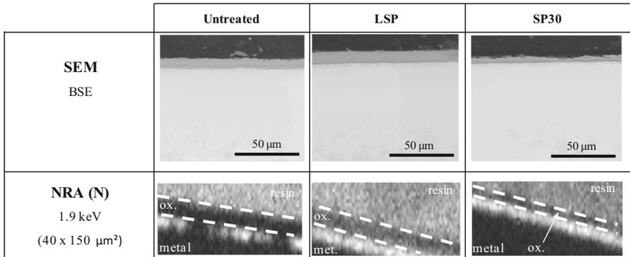
**Fig. 5** Comparison of samples after oxidation under dry air at 700 °C. In SEM images, the *black upper part* is the coating resin. For the NRA images, the oxide is located between the *white dashed lines*, and the metal is under the *lower line*
