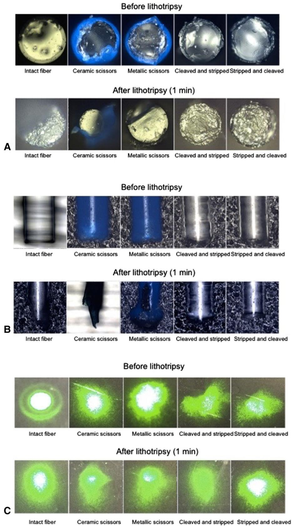
Cleaving the laser fiber systematically has been recommended with the intention of regaining the efficiency of a fiber damaged by mechanical and thermal burn-back effects of lithotripsy [3, 11].
