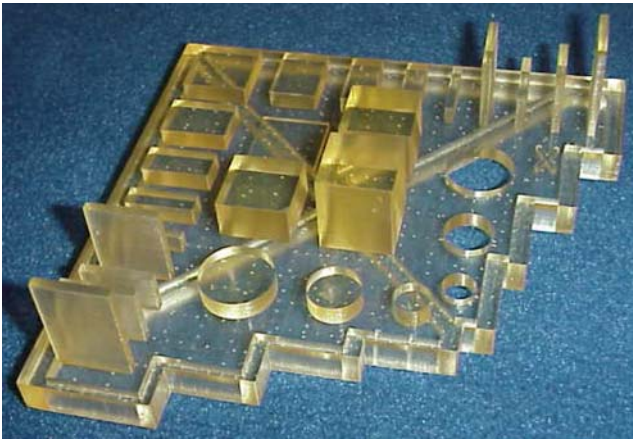
Fig. 4 Resin test part realized by laser stereolithography
