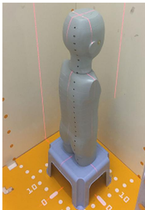
Fig. 1 The anthropomorphic phantom, representing a 5-year-old child, placed in posterior-anterior-lateral positioning within the EOS scanner
