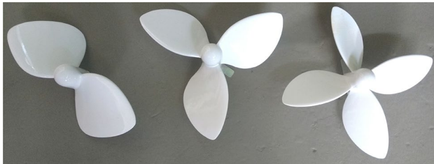
Fig. 6 Small-scale runners with two, three and four blades
