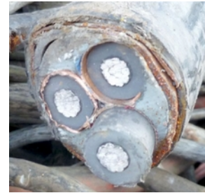
Fig. 2. Section of multiple aluminum beams cable
