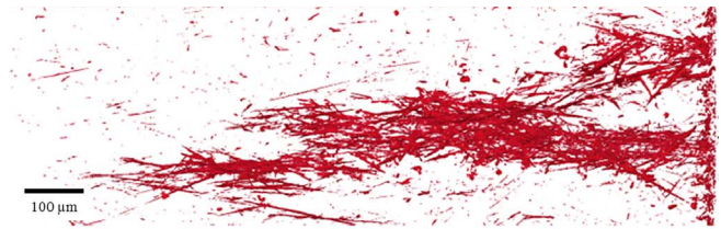
(b) Damage (fibers oriented at 90°)
