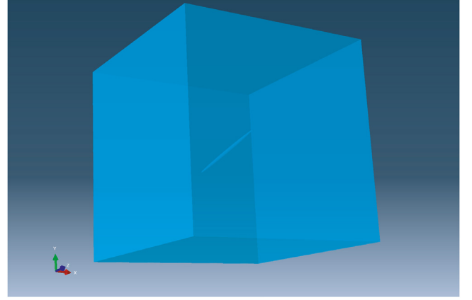
Fig. 6. The cubic volume (shown translucent) meshed for the study of the rotation of a tilted prolate spheroid (shown in light color). A simple shear is applied, which translates the upper and lower faces of the cube in opposite directions.
