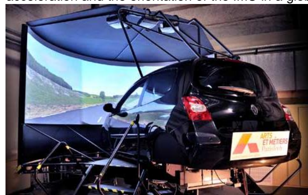
Figure 1. SAAM: hexapod driving simulator
