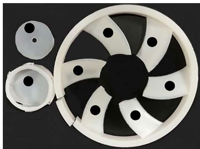
Fig. 7 Thickness measurement locations
