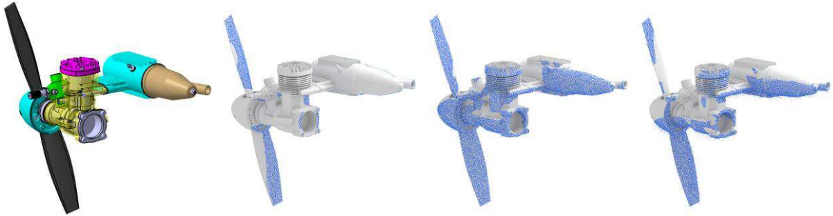
Figure 9: CAD model of a RC engine reversed engineered with configurations 1 to 3.
