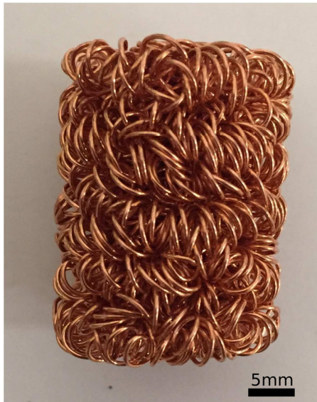
Fig. 1. Picture of single copper wire entangled sample.
